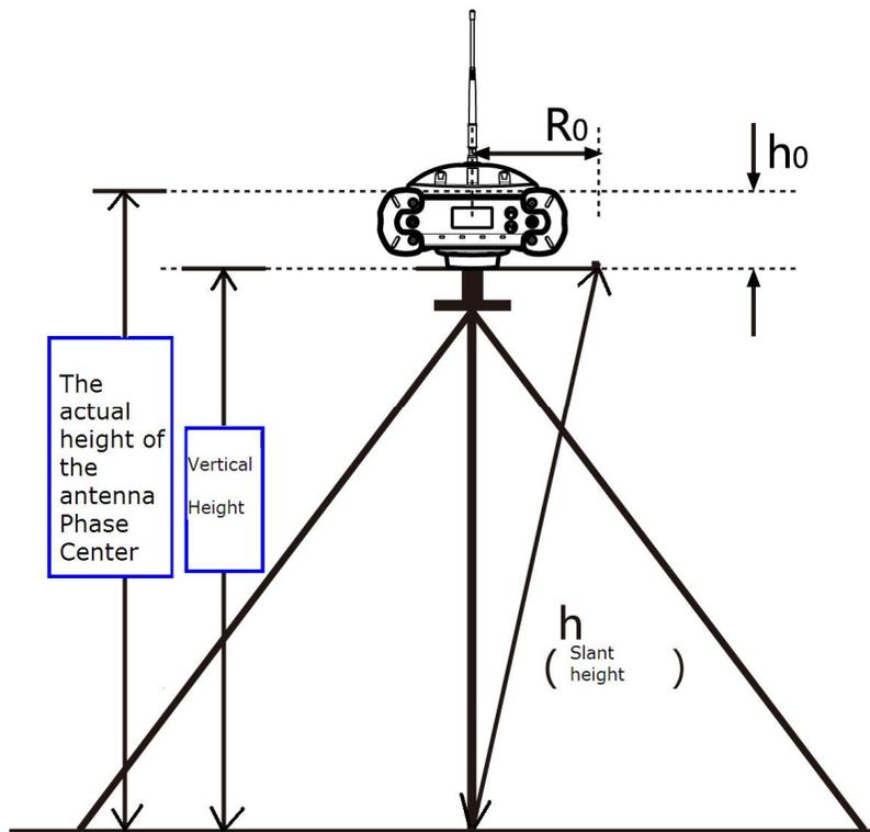
The antenna height measuring for K300
