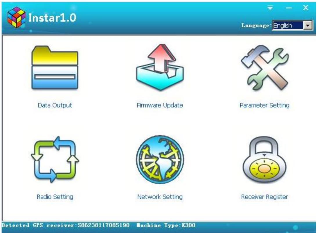
Go into Data output, you can see the data stored in the receiver. Select the data you need and output target, then you can output the data in DAT format or in Rinex format
