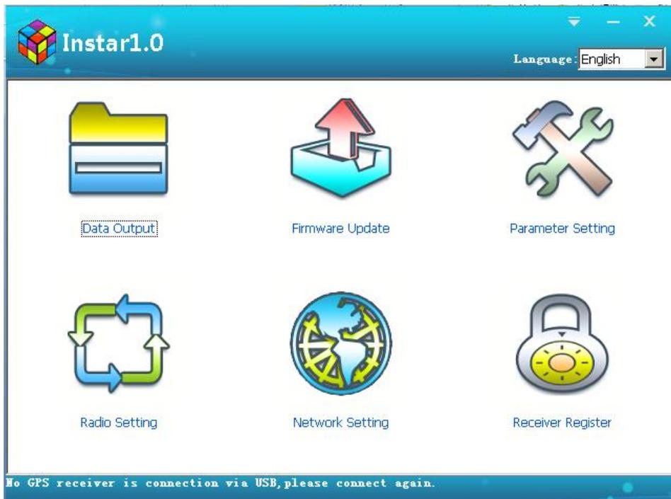
Data output: to copy static data from receiver (USB port);
