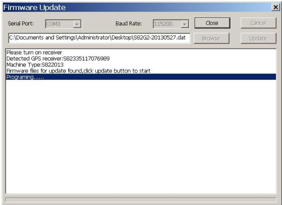
Select the right port and baud rate 115200, open, then power on the receiver
