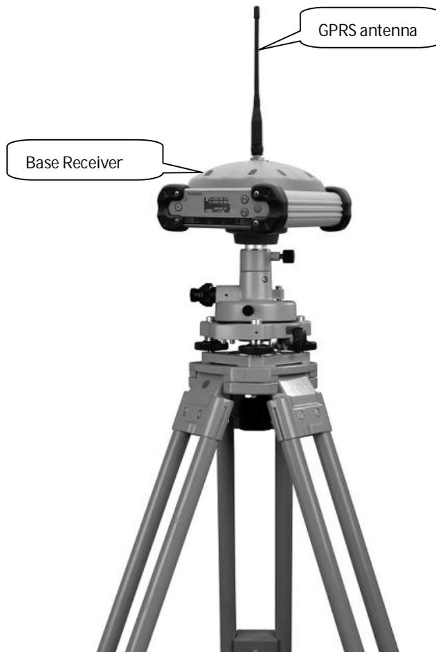
Built in GPRS or GPRS/3G module Base Station
