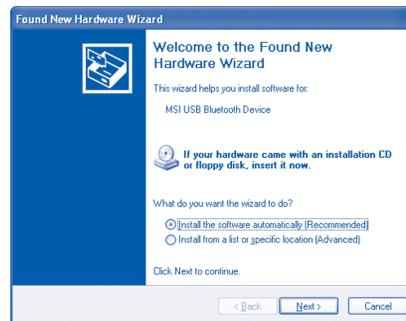
7. After the Bluetooth USB adapter is connected, click **Next** to install the driver software.
