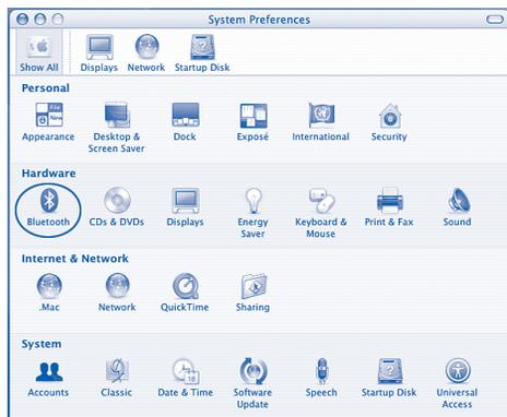
With the Bluetooth USB adapter plugged in, go to System Preferences to adjust your Bluetooth configuration.
