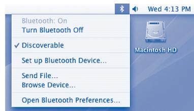
After you plug in the Bluetooth USB Adapter, a Bluetooth icon appears in the upper-right corner of the Finder Menu. Use this menu to set up other Bluetooth devices, send files to paired Bluetooth devices, or open the Bluetooth System Preferences pane.
