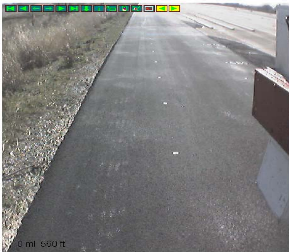
Figure 18. Typical PAVECHECK Video Image with Menu Options.
