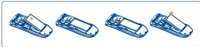
Insert and click the battery into place, then close the telephone cover. Unclip the cover, then remove the battery.
