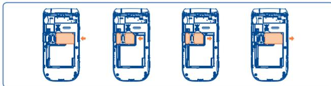
Place the SIM card with the chip facing downwards and slide it into its housing. Make sure that it is correctly inserted. To remove the card, press and slide it out.
