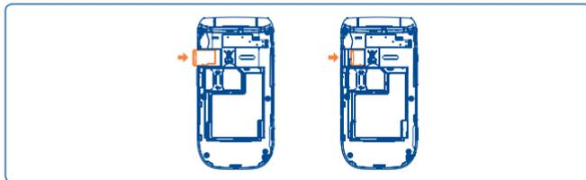
Insert the microSD card with golden contact facing downwards into the slot until it is locked. To remove, gently push the memory card until it is unlocked.
