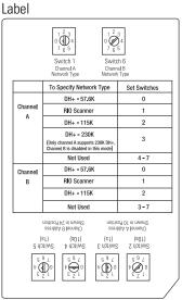
If you set the network type to Data Highway Plus (DH+), also set the node address switches for that channel to a unique address within the range of 0...77.
