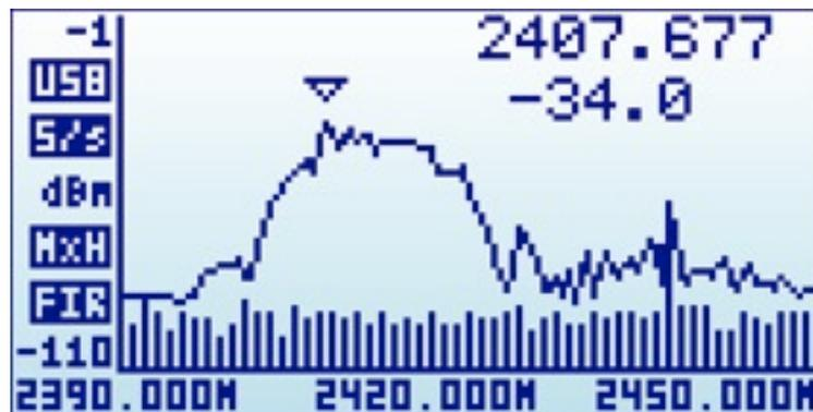
The X axis represents frequency in MHz and the Y axis represents actual received power (amplitude) in dBm or dBuV.
