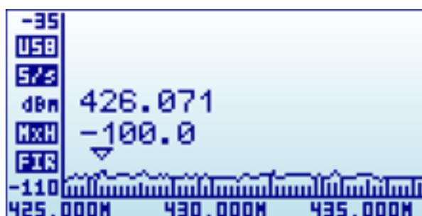
**Note:** While RackPRO Spectrum Analyzer screen is enabled, the [Left] and [Right] buttons can be used to increase or decrease the Start/Stop frequency, virtually moving the visible spectrum to
