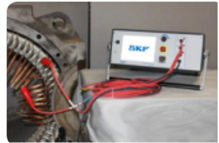
**A Baker DX-15 testing individual stator coils.**
