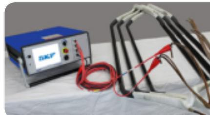
**The Baker DX-15 as a coil test analyzer.**
