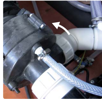
Check pump connections (4), make sure these are water-tight, to prevent possible leaks into the equipment compartment.
