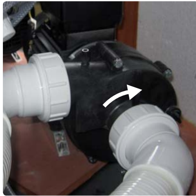
Check pump connections (4), make sure these are water-tight, to prevent possible leaks into the equipment compartment.
