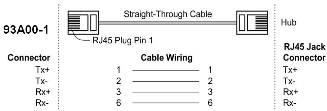
Connect the 10/100 Port on the 93A00-1 to an Ethernet card using a crossover network cable.
