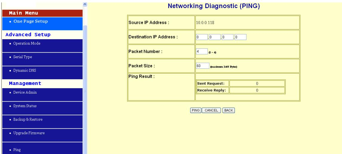
**Source IP Address:** the current IP address of the 93A00-1 (read-only).
