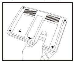
**Initial Charge:** The Li-Ion batteries are approximately 60% charged prior to shipping. Before first use batteries should be charged 8 to 12 hours. During this initial charge, please continue charging even after the LED charge indicator light turns to green.
