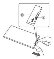
• Place a new battery in tray, and re-insert the tray making sure the (+) mark is facing upwards.
