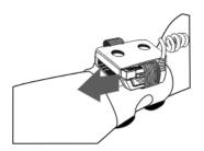
1. Slip the ring cable connector through the elastic ring cable guide on the side of the Bluetooth module sleeve. The connector can be inserted from the left or the right. The ring cable guides are designed to minimize excessive pulling or tugging on the scanner cable after the ring device is connected to the Bluetooth module.
