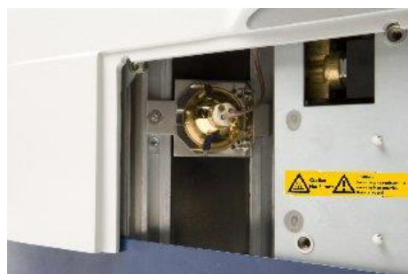
Lamp access panel removed
