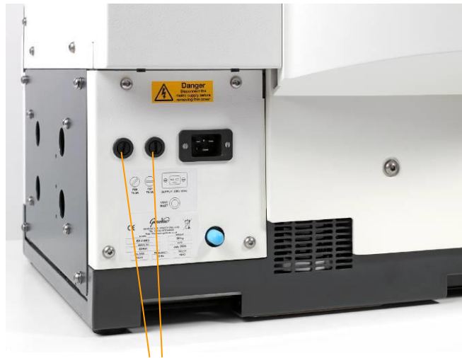
Mains inlet / outlet fuses
