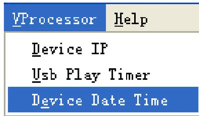
Remember to set the Device Date Time to the same to the local time, and after set, can check also on the front panel LCD module.
