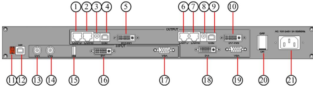
1,2,6,7: Gigabit copper port, connect to LED screen;
