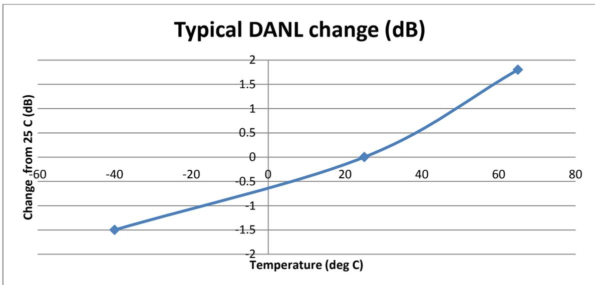
\* Shown for gain 3, attenuator 0 dB. For auto gain/attenuator settings at cold temperatures, a reference level of -55 dBm may be required for maximum sensitivity, instead of the usual -50 dBm.
