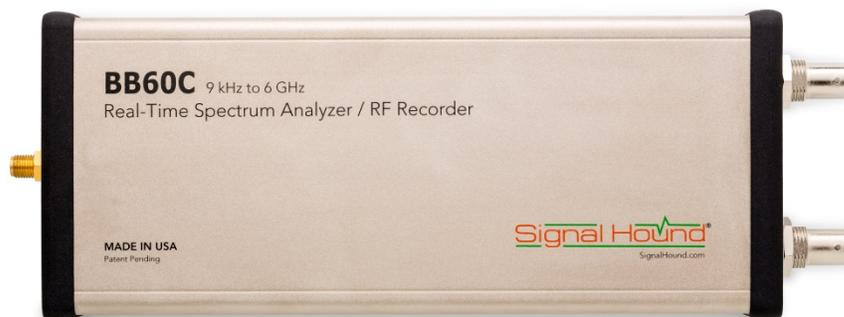
Super Speed link. It has 27 MHz of real-time bandwidth, tunes from 9 kHz to 6 GHz, collects 80 million samples per second, and streams data to your computer at 140 MB/sec. By adding a high speed hard drive to your PC or laptop (250 MB/s sustained write speed), the BB60C doubles as an RF recorder, streaming up to 80 million IF samples per second, or 40 million I/Q samples to disk.
