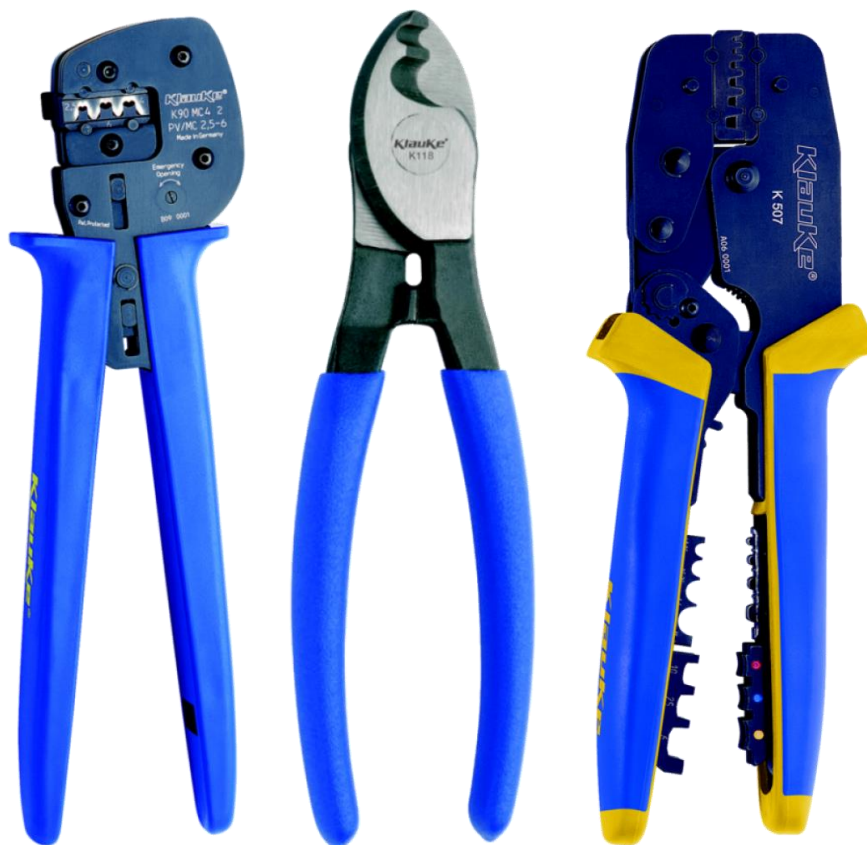
Figure 5.5. Examples of the needed hand tools for the PV cable connectors and water level sensors cable connectors.
