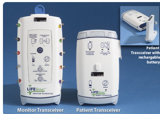
Figure 8- The patient transceiver (sensor unit) and monitor transceiver (receiver unit) of the LifeSync Wireless ECG System [11].
