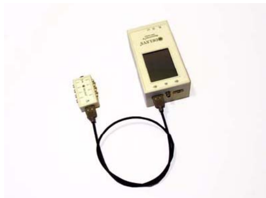
Figure 4- The Myomonitor wireless EMG module connected to the input module [7].
