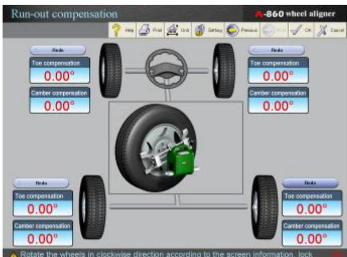
level and the wheels are hanged in the air. Press [Next] after finished to perform run-out compensation, the screen will display the following interface.
