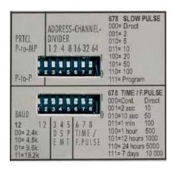
The channel must be same for both C-LINK 100 units before turning the power ON. When the power is turned ON the operational channel has been selected.
