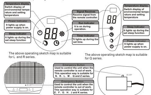
**Remarks:** When remote controller is out of work, open the panel and you can see emergency button there, see the above pictures. The emergency button for 15K、16K、18K、22K、24K and 30K series is at the top right, see "ON/OFF" button there.
