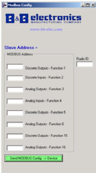
The Modbus configuration menu will allow you to adjust the base address for the I/O to be displayed or controlled. When in Modbus mode, the radio ID number is within the Modbus configuration menu.
