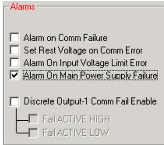
The RT series RTU's have several types of alarms. Below is a description of each alarm. To modify or change any of the alarms, click on the respective box or boxes, and press the "Send Parameters To Device". Make sure you are "Connected". Alarms are local to the RTU. Each RTU has a built in beeper alarm. Most alarms will sound at the master as well as the slave units. Most of the alarms apply even in Modbus mode.
