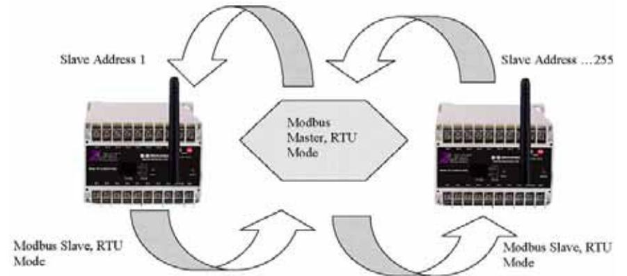
This typical application shows two Slave Modbus controllers. Modbus slave controller can be address from 1 to 255.
