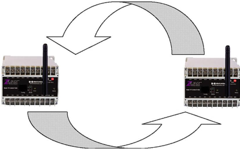
This typical application shows the INPUT voltage signals from the Master controller is sent to the Slave controller. The save output voltages reflect the Masters input voltages.
