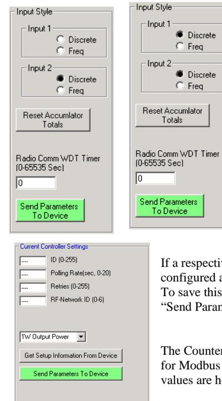
The RT series RTU's support the ability to configure DI-1 and DI-2 as Digital or Frequency/Accumulator inputs. Some RTU have an additional, dedicated, "Freq" input.
