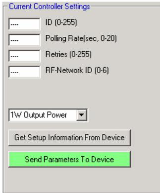
**Retries:** In Peer-to-Peer mode, this parameter determines the number of consecutive failed polling attempts before a communications failure occurs. It is not recommended to set the number of retries higher than 10 attempts. Large numbers may cause an unnecessary delay in communications failure response time; a low number may cause the system to prematurely fail. This parameter has no affect in Modbus mode.
