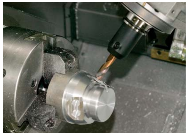
Machining in the tilted plane
