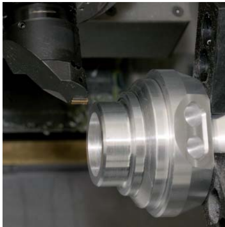
... longitudinal turning with the same tool ...
