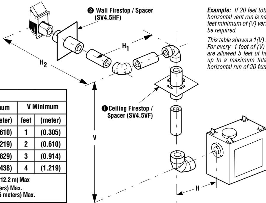
**Example:** If 20 feet total ( $H+H_1+H_2$ ) horizontal vent run is needed, then 4 feet minimum of (V) vertical vent will be required.
