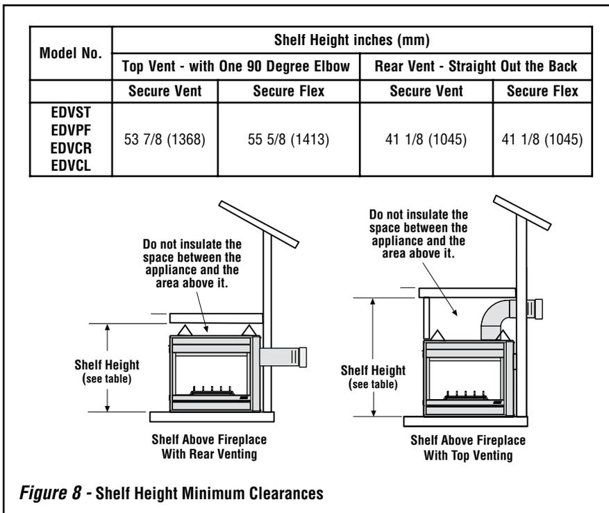
Figure 8 - Shelf Height Minimum Clearances
