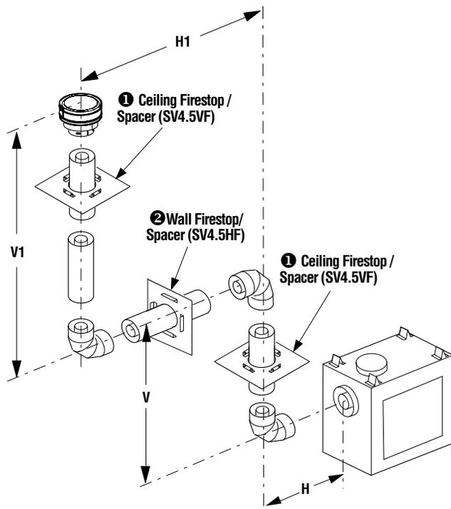
**Figure 38 - Side Vent - THREE ELBOWS**
