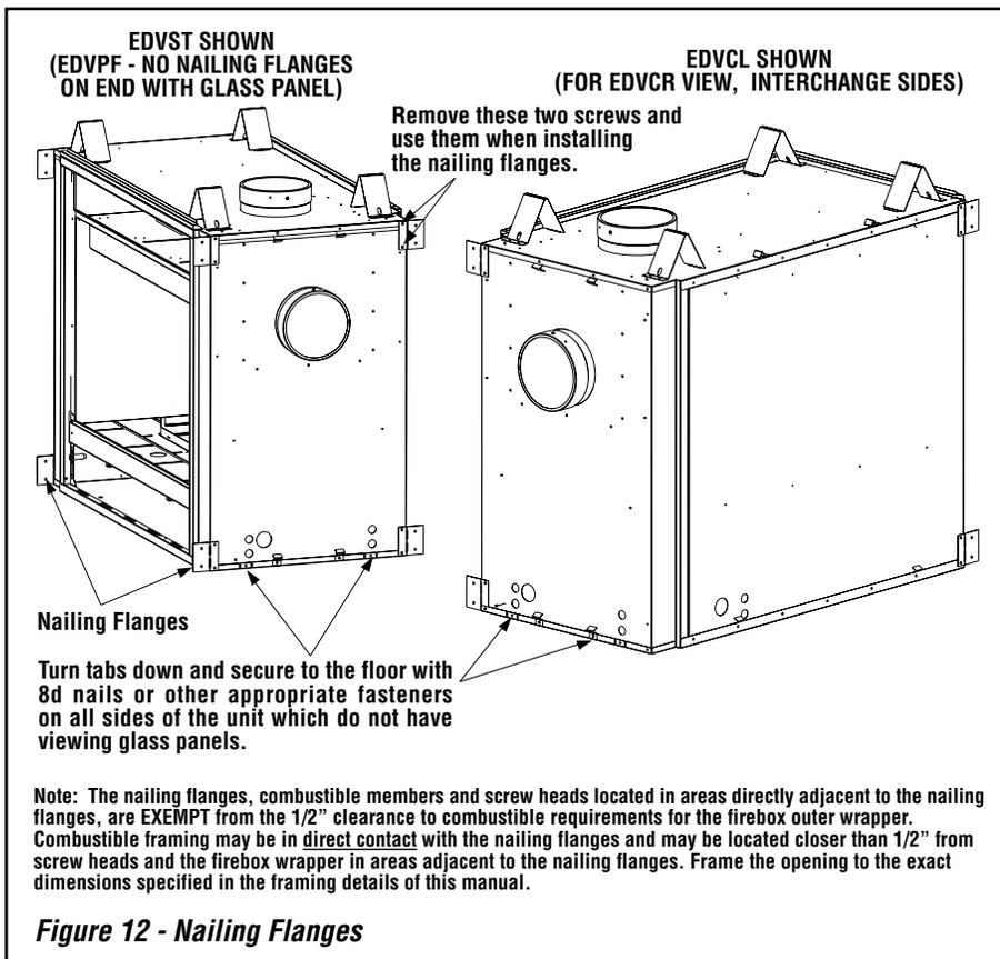
Figure 12 - Nailing Flanges
