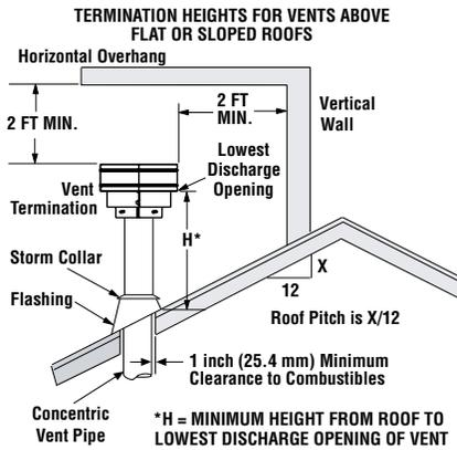
The vent / air intake termination clearances above the high side of an angled roof is as shown in the following chart:
