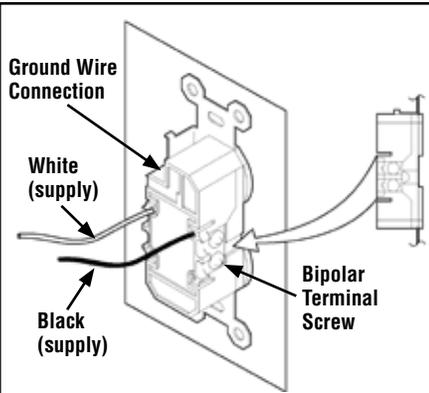
**Note:** Supply wires may be alternatively connected to the outlet using the screw terminals, however the black supply wire must be wired to a terminal that is opposite (across the outlet) the point where the white supply wire is connected.
