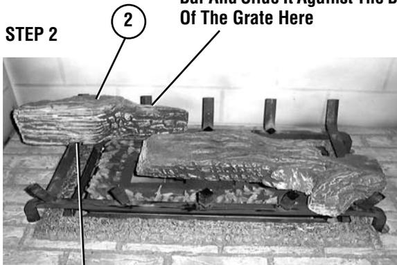
Position Groove At The Bottom Of Log (2) Over The Grate Here And Slide It Against The Back Of The Grate
