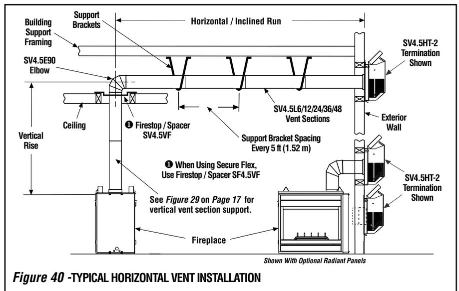
The unitized design of the **Secure Vent** components will engage and seal both the inner and outer pipe elements with the same procedure. Sealant and securing screws are not required.
