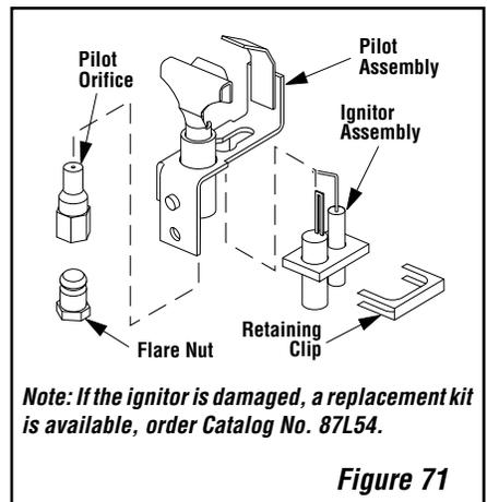
**Note: If the ignitor is damaged, a replacement kit is available, order Catalog No. 87L54.**
