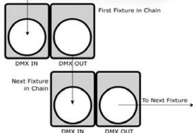
**Step 3:** Connect other fixtures in the chain from output to input as above. Place a DMX terminator on the output of the final fixture to ensure best communication.
