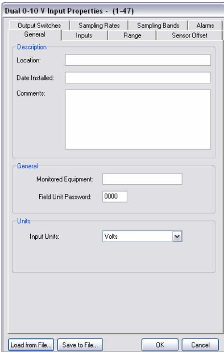
Figure 4.6: Password Setting Using Wireless Instrumentation Manager
