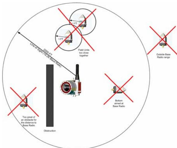
Figure 3.1: Examples of Incorrect Field Unit Positioning
