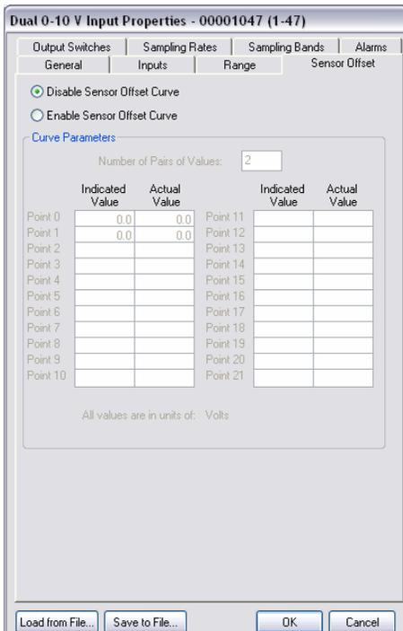
Figure 7.5: Setting a 22-Point Curve Using Wireless Instrumentation Manager
