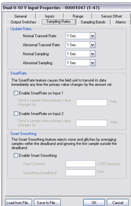
Figure 6.9: Smart Rate Configuration Using Wireless Instrumentation Manager
