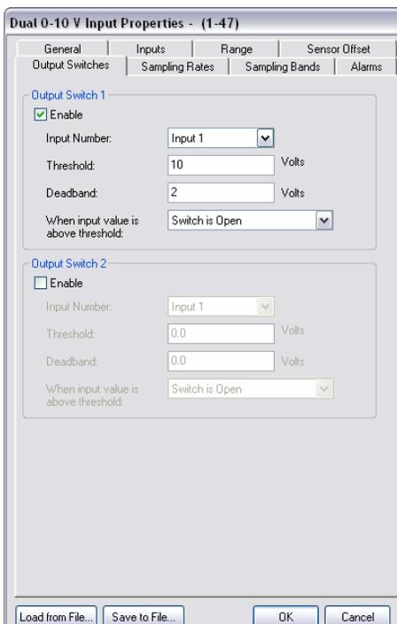
Figure 3.6: Output Switch Configuration Using Wireless Instrumentation Manager
