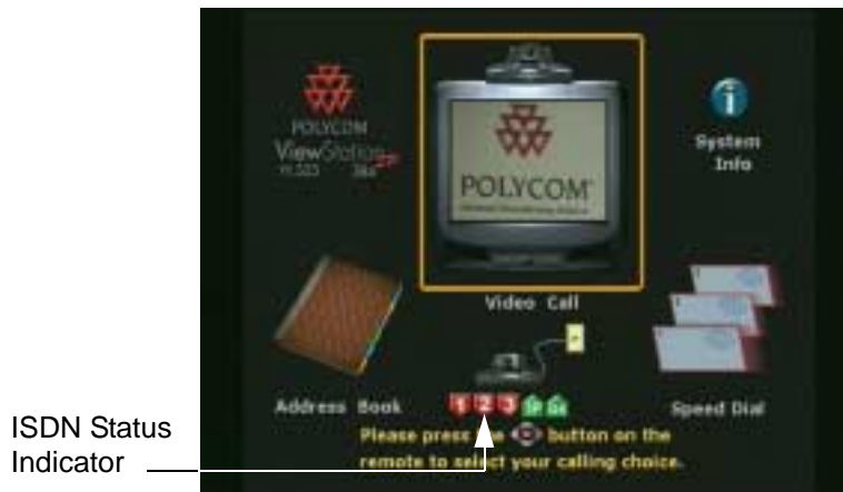
Figure 3-2. ViewStation SP384 Main Calling Screen
