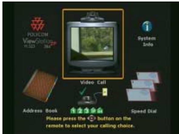
Figure 3-3. ViewStation SP384 Main Calling Screen
