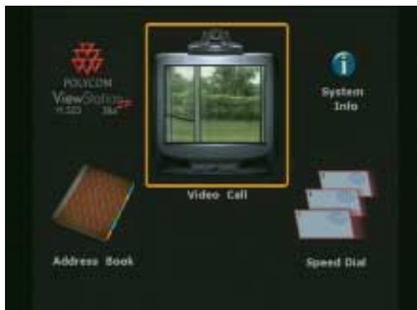
Figure 3-1. ViewStation SP384 Main Calling Screen
