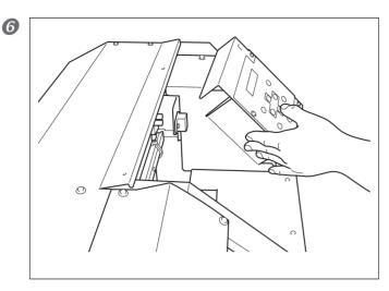
Touch the location shown in the figure to discharge any static electricity.
