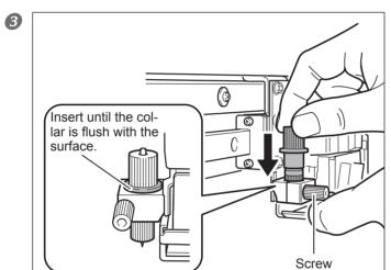
Support the screw from below and insert the blade holder.
