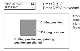
If the printing and cutting lines are aligned, adjustment is complete.
