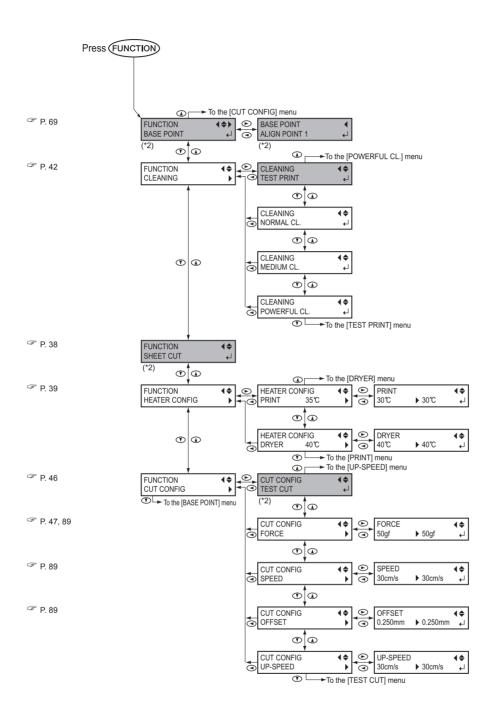
(\*2) This is not displayed when no media is loaded (that is, when SETUP is dark).
