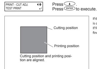
If the printing and cutting lines are aligned, adjustment is complete.
