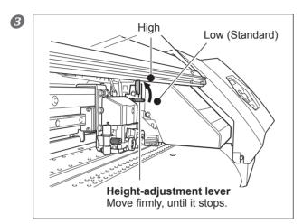
Open the front cover. Move the height-adjustment lever to adjust the head height.
