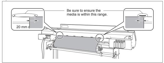
Secure the stoppers in place in alignment with the width of the media.
