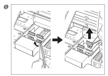
Detach the old wipers. Detach the hook and pull up and out.
