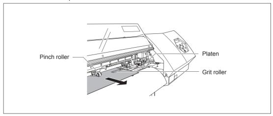
**6** Make sure both edges of the media are above the grit rollers, then place pinch rollers over all grit rollers covered by the media.
