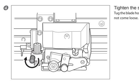
Tighten the screw. Tug the blade holder upward to make sure it does
