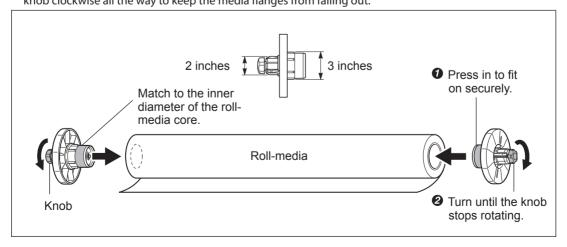
3 Place the roll media on the shafts and position its left and right edges to match the grit patterns.
