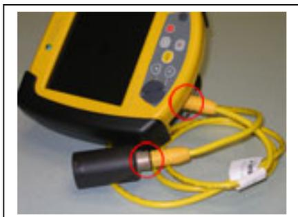
Step 8: Connect cable to Display Unit & Camera Head
