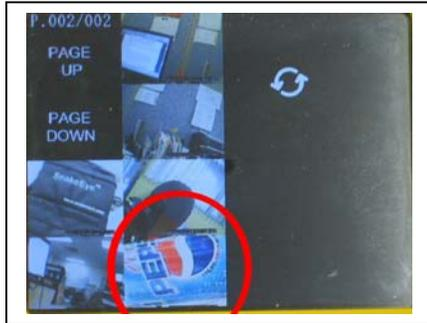
Every time the user selects the “PHOTO PLAYBACK” function, the cursor will always point to the last image taken, and the user can use “UP” and “DOWN” arrow keys on the postproduction keypad to move the cursor to the image that the user would like to review. Pressing the “Enter” key will enlarge this image to a full-screen image. While in full screen mode, the user can press “UP” and/or “DOWN” key to browse the previous/next full-screen image.
