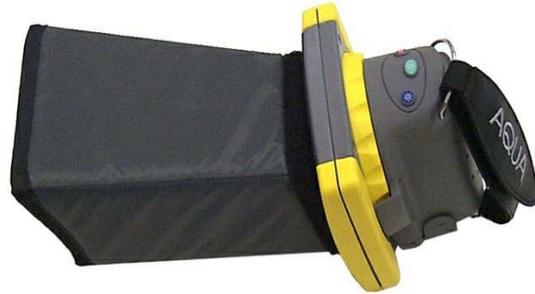
The Sunshield is attached by folding into a rectangular shape as shown in the photograph.
