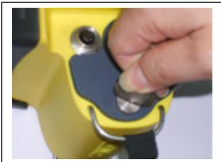
Step 3: Mount the Access Cover and use coin/fingers/screw driver to tighten two screws
