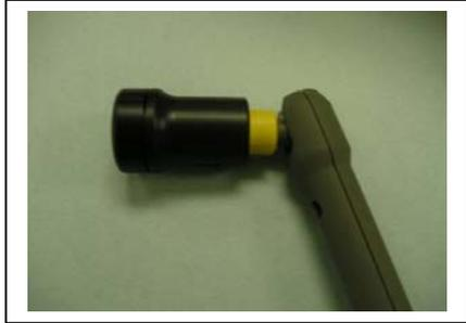
The Extension Wand is designed to extend the effective operating range of the unit. This accessory comprises a rigid handle, unidirectional swivel mount and a sliding switch which controls the angle of the Camera Head (from 0° to 90°) in the swivel mount. Under most conditions, the Extension Wand provides the greatest operating flexibility.
