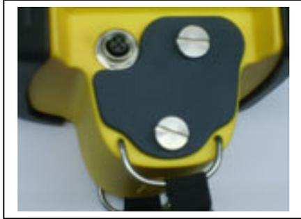
Step 4: Ensure the Access Cover is properly installed for dustproof/waterproof.
