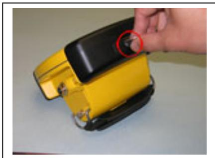
Step 7: Install SD Card Cover & Tighten Screw
