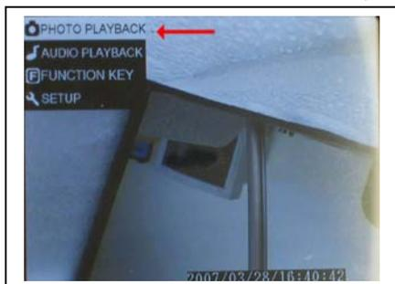
1. Review the images recorded by selecting the “Photo Playback” on-screen-command. **In the “Photo Playback” mode, the screen will display up to sixteen index icons (including “PAGE UP”, “PAGE DOWN” icons, and fourteen image index icons) on the LIFO (Last-In-First-Out) basis.**
