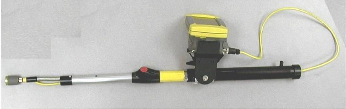
Camera and Display mounting platform to extend the viewing reach of SnakeEye. Each pole has multiple extension locking positions spaced at six-inch intervals. The pole may be rotated within the handle to give 360° viewing. The camera head may be articulated 130° from the straight position.
