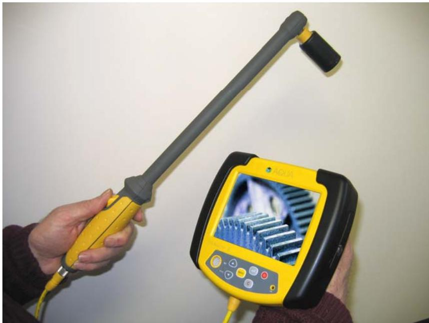
The SnakeEye™ III records images as snapshots (Page13) that are stored on a removable SD (Secure Digital) card or, when connected to a VCR, as streaming video (Page 21).
