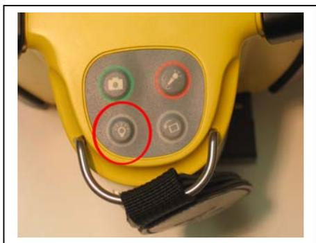
4. Turn on/off and adjust three intensity levels of the light source on the camera head by pressing the “Camera Light Source” button on the operational keypad. Pressing the “Camera Light Source” button will toggle the camera lights through the Low, Medium, and High Intensity and then Off cycle.
