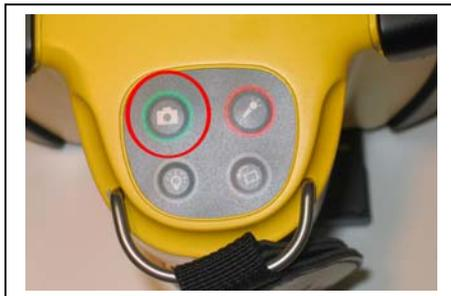
1. Record still pictures. Pressing the “Snapshot” button on the operational keypad, the SnakeEye III will store the “current displayed image” onto the SD card after first checking for available space on the SD card. The user will briefly see the recording symbol and the amount of space available on the SD card at the right-top corner of the display screen.
