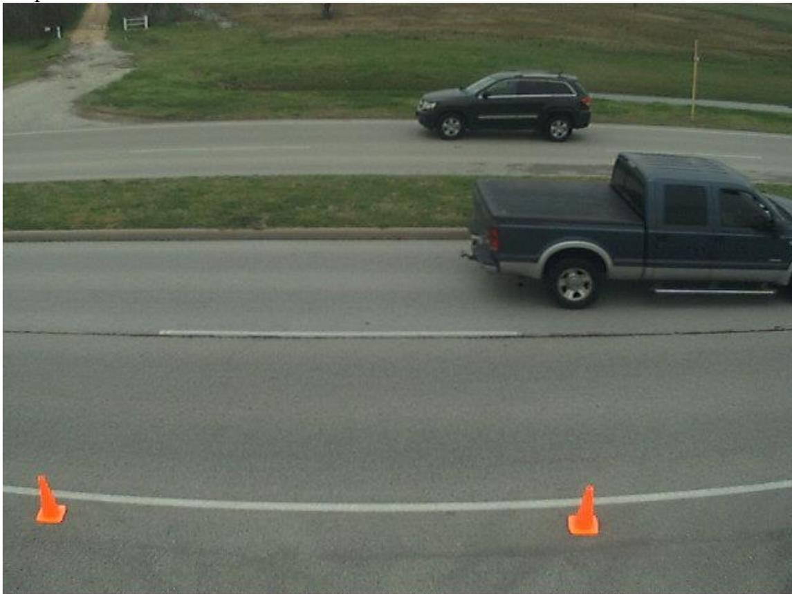
An example photo from the SpeedLane sighting camera showing proper pointing for a 4 lane highway.
