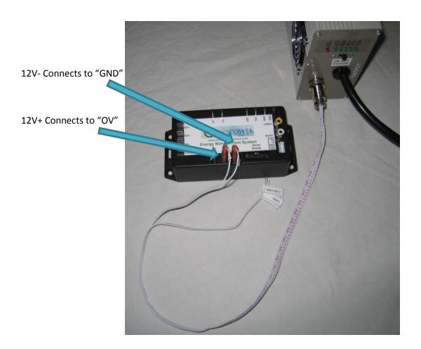
For a CAN communication connection connect the CANH, CANL and CAN GND to the matching connection on the CAN connection on the EMS CPU. The white connector may be cut off of the cable; however, note which wires are which before doing so.
