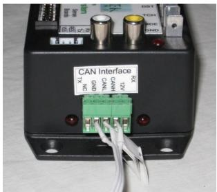
If both the CAN communication and the digital inputs are connected CAN communications will take priority over the digital input for charge control. CAN communications requires the optional CAN board be installed on the EMS CPU.
