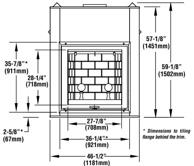
Figure 15 - Framing Dimensions
