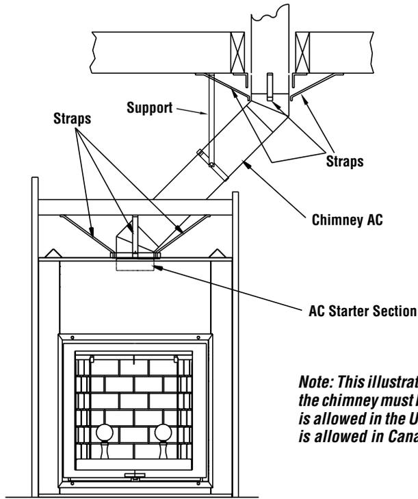
*Note: This illustration is not to scale. It represents how the chimney must be supported. A 30 degree offset only is allowed in the USA and a 45 degree maximum offset is allowed in Canada.*
