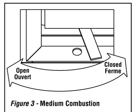
Figure 3 - Medium Combustion
