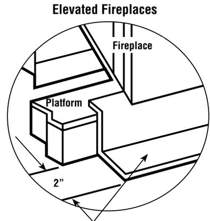
Elevated fireplace installations require a special "Z" Metal Safety Strips (field provided), in place of the safety metal strip shown above. The safety strip should extend the full width of the fireplace. When more than one safety strip is used they must overlap by a minimum of 1".
