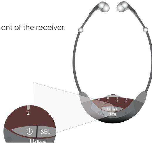
**ATTENTION 1:** The LR-44 model must have a headset connected to the unit to turn on and remain on for longer than ten seconds.
