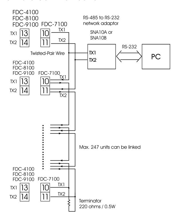
Figure 2.19 RS-485 Wiring
