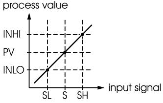
Figure 3.1 Conversion Curve for Linear Type Process Value
