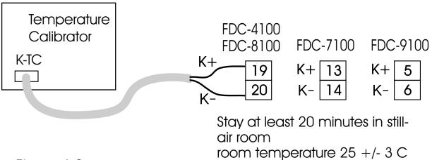
Figure 4.2 Cold Junction Calibration Setup
