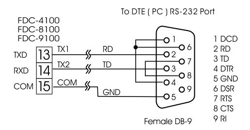
Figure 2.21 Configuration of RS-232
