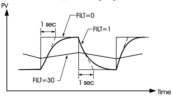
Figure 3.8 Filter Characteristics
