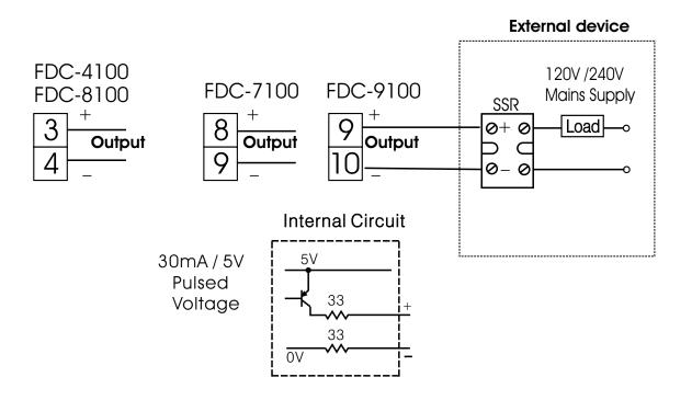
Figure 2.10 Output 1 Pulsed +5 VDC Voltage to Drive SSR
