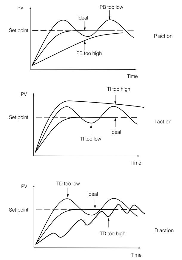
Figure 3.9 Effects of PID Adjustment
