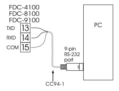
Figure 2.20 RS-232 Wiring
