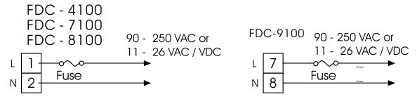
Figure 2.7 Power Supply Connections
