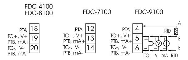
Figure 2.8 Sensor Input Wiring
