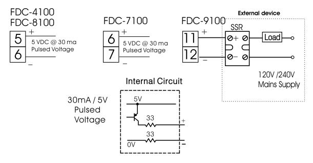
Figure 2.14 Output 2 Pulsed Voltage to Drive SSR
