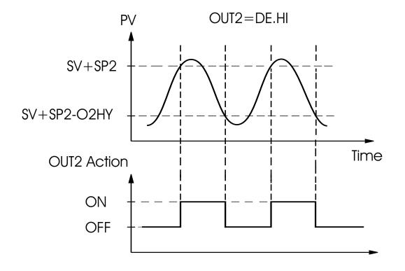
Figure 3.3 Output 2 Deviation Time High Alarm
