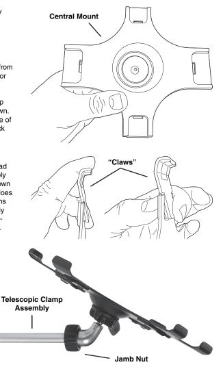
4) Use the "C" clamp to mount the iMS-1 to a mic stand, desk, headrest, or any surface up to 1 in. thick.
