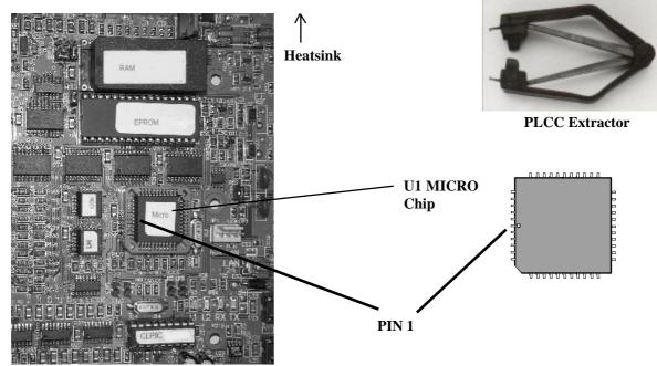
Section of the Model 3000/ Access 4000 panel PCB
