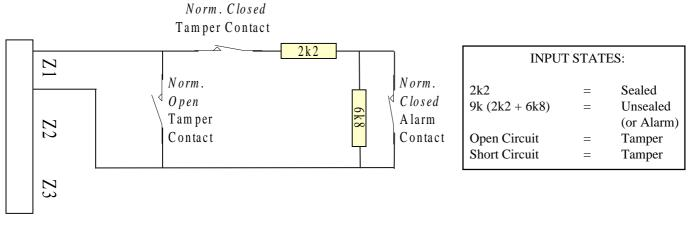
Detection devices with *Normally Open* Alarm contacts are wired in exactly the same manner as above. When programming the Zone Input, however, the option to "Swap Seal and Alarm conditions" must be set to [Y]es.
