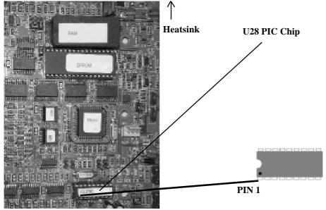
Section of the Model 3000/ Access 4000 panel PCB
