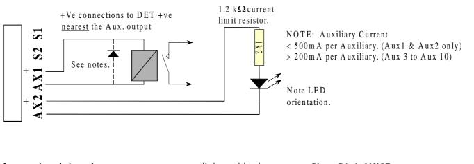
Locks are activated via a relay. External power supply is used for lock power to prevent voltage spikes reaching the Concept equipment, provide longer battery backup & minimise the possibility of earth loops.
