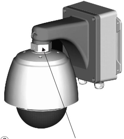
• Seal this using the Teflon tape around a thread of a socket.
