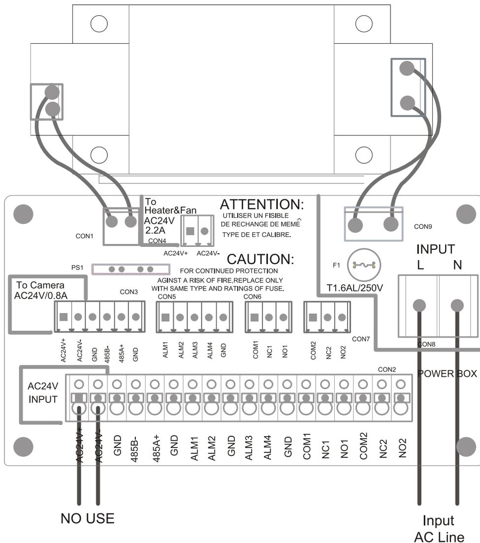
CON4 : for one Heater and one fan with AC24V
