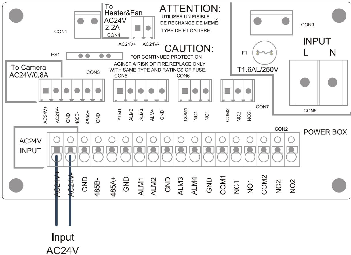
CON4 : for one Heater and one fan with AC24V
