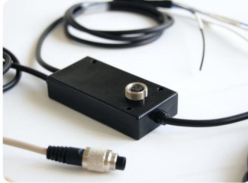
To connect **ECU Bridge** (RS232/CAN) using a direct connection it is necessary to connect the free cables to ECU pinout.
