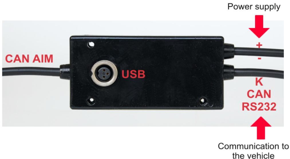
Here above the **ECU Bridge** is shown, with its connector and three cables (two on the right and one on the left side).
