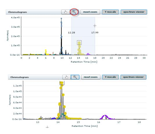
The *Y rescale* button, when active (default) allows automatic rescaling of the Y axis of the zoomed Chromatogram at all magnified states to the max y value of the current zoomed in region. Inactivate it to leave the y axis scale to the full Chromatogram range.
