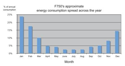
Increasing the indoor temperature one degree increases power consumption by approx. 5%.
