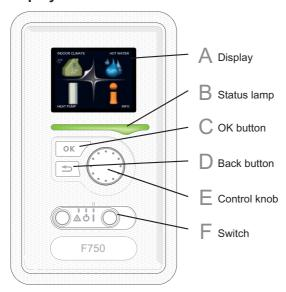
There is a display unit behind the heat pump door, which is used to communicate with F750. Here you:
