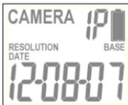
***If no buttons are pressed after 30 seconds the LCD screen will power down to conserve battery life and enter 1 minute count down to enter PIR detection mode. To re-power the display screen, press and hold the UP or DOWN button until you see the status screen.***
