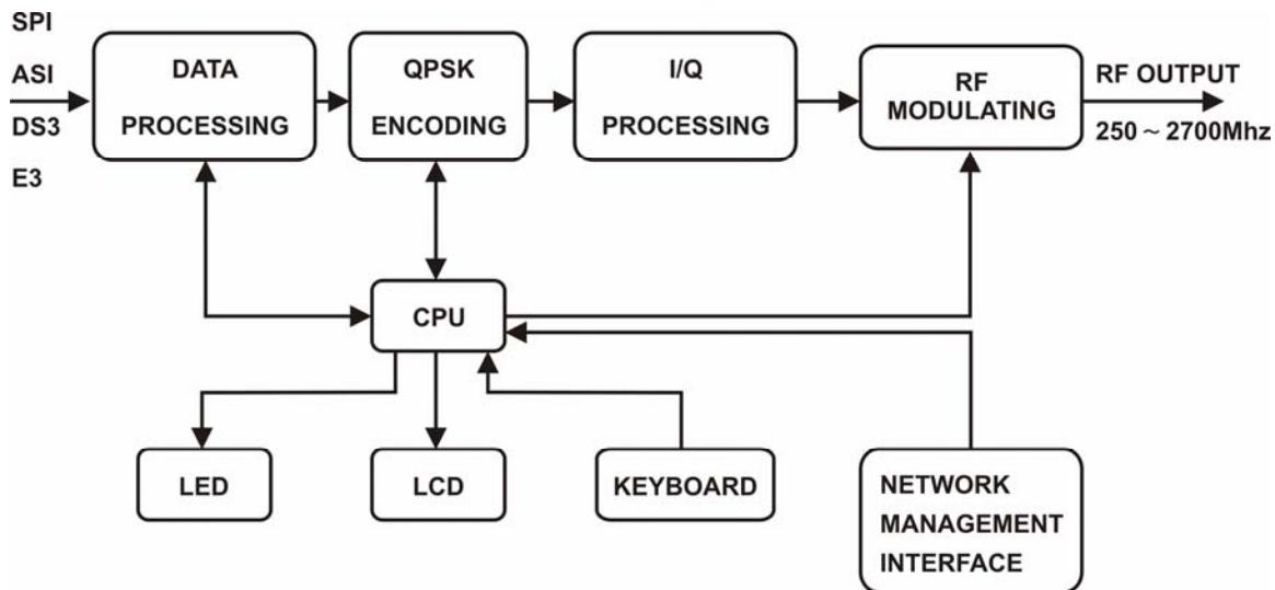
QPSK Digital Modulator is mainly composed of the following modules:
