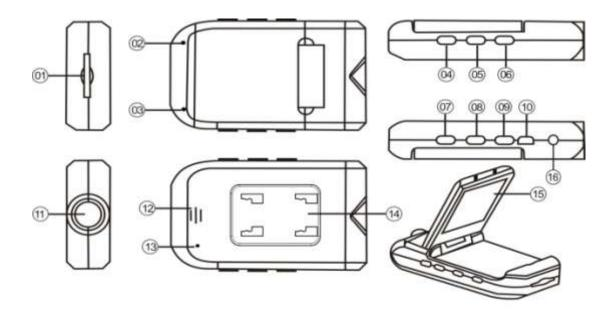
9. MODE switch modes button (recording/photo/preview) 1. Memory Card slot 2. Indicator light **10.USB** Interface 3. Microphone 11. Lens 4. REC/SNAP: Confirm/Select button 12. Speaker 5. MENU 13. RESET 6. POWER: Day/Night Mode 14. Bracket slides 7. DOWN: Flip Screen (must use firm pressure) 8. UP: Flip Screen 15. 2.5 inch LCD screen 16. AV OUT: AV output interface
