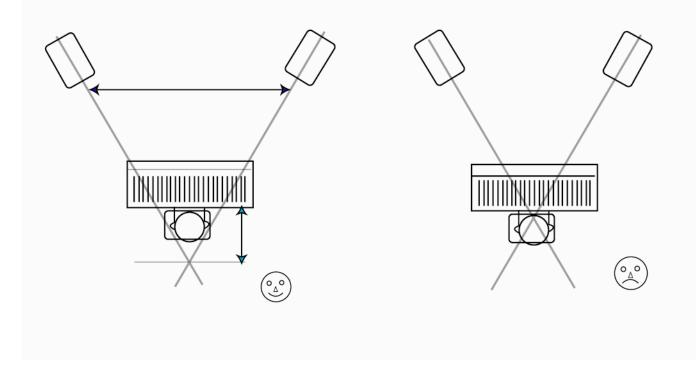
The height and angle of mounting the speaker is equally as important. The correct height and angle should result in the axis being at ear level when the engineer is sitting in his normal position at the console.
