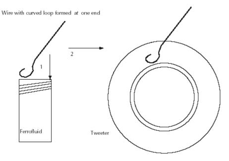
Dip wire in ferrofluid, a small amount will be retained on the wire hold wire over the tweeter gap and the magnet will attract the fluid from the wire into the gap. Do this 3 or 4 times in different position on the tweeter, then check by inserting the new diaphragm to see the amount of fluid in the tweeter.
