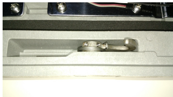
Figure 9 Position of Latch CAM and Southco Spring assembly
