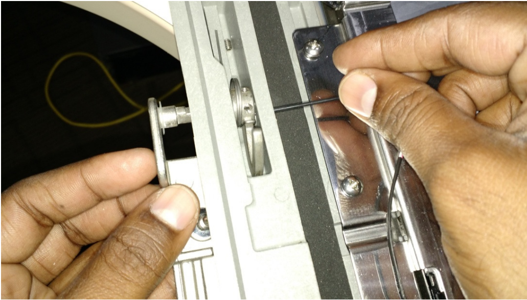
Figure 3 — Removing both the hex nuts
