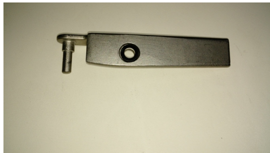
Figure 4 Adding C shaped washer
