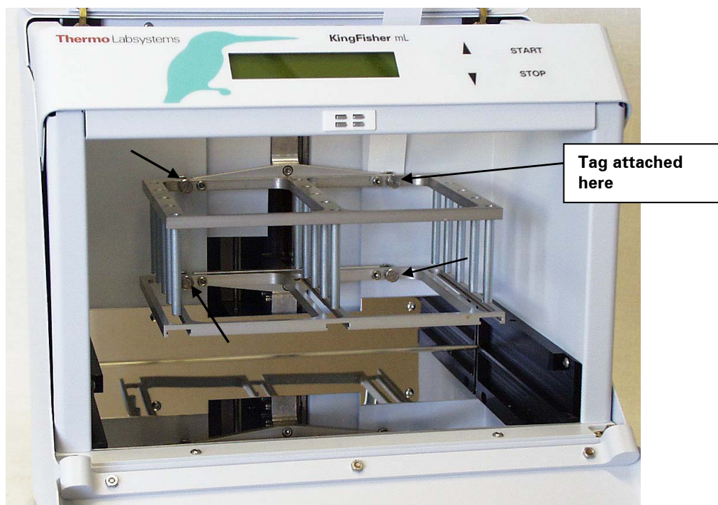
Fig. 5.2 Location of the transport lock screws and warning tag
