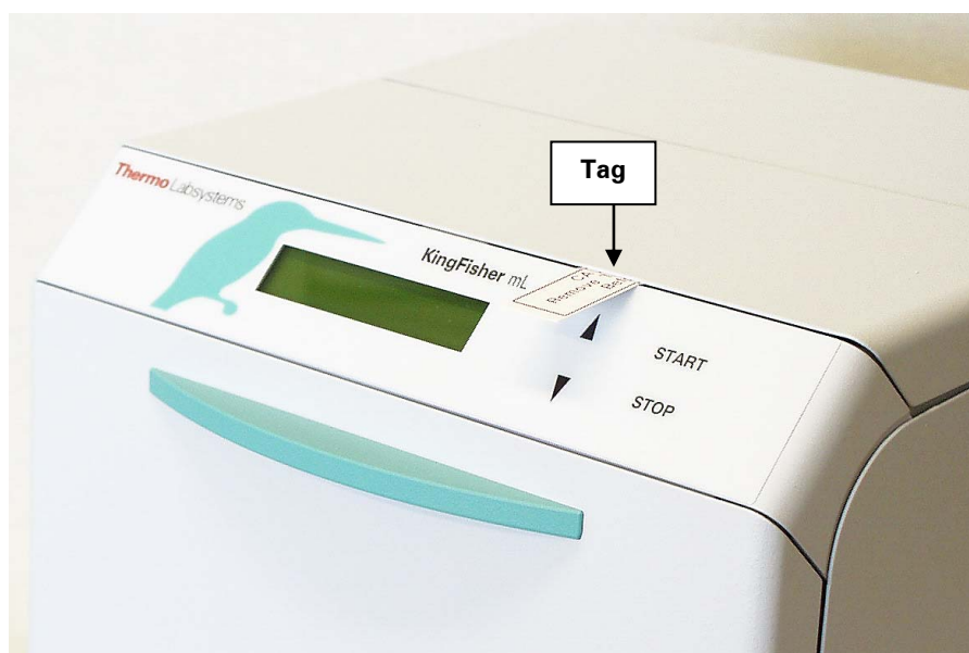
Fig. 5.1 KingFisher mL transport lock tag present before release of the locks
