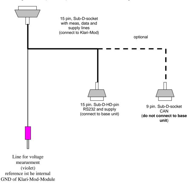
During installation you connect the violet meas line with the voltage to measure (e.g. pluspole of the battery in vehicle). 15 pin Sub-D-HD-pin you connect to the socket on the right side of the base unit.
