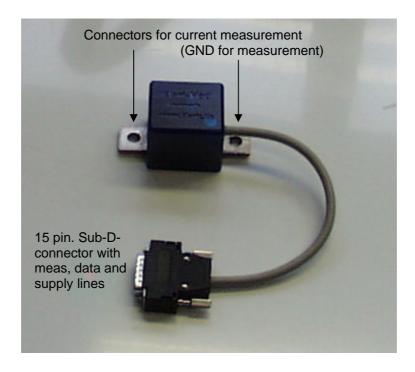
With the two connectors the current meas module will be inserted into the current loop. There are different adapters available (pole connectors, brass poles, cable lug). Note that the left connecter where the cable comes out represents the internal GROUND potential.
