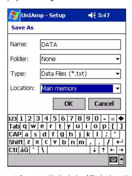
In this window you define the root directory with the help of fileds "Location" and "Folder". With "Location" you select the storage device, e.g. main storage of PDA, CF-Card or SD-Card. With "Folder" you can specify optionally a subdir in these storage devices. You have to notice that Klari-Amp-Software will create date related subdirs by itself.
