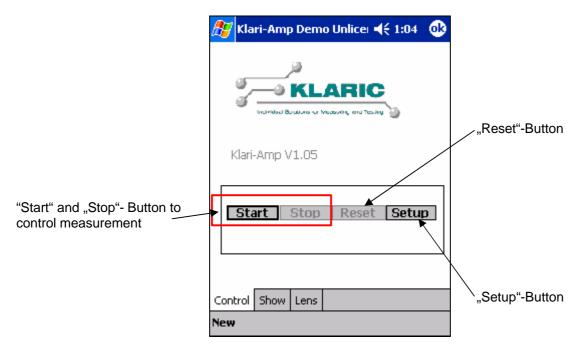
Using "Start"-Button a measurement is started. A new meas result file will be created and header lines defined in "Setup-Data" are inserted. After that for every new measurement a new line will be appended The received meas values are displayed on screen. Note that the display is not so fast like the real storage. During recording no setup data could be changed. "Setup"-Button is deactivated. A running measurement recording is visualized by a black background of the "Start"-Button.
