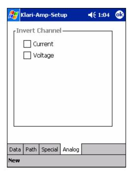
With this checkboxes it is possible to invert the analog channels, i. e. change the sign of the values.
