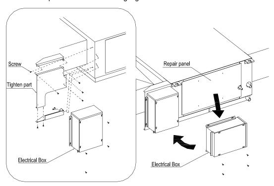
Fig. 21 Schematic for the Electrical Box part
