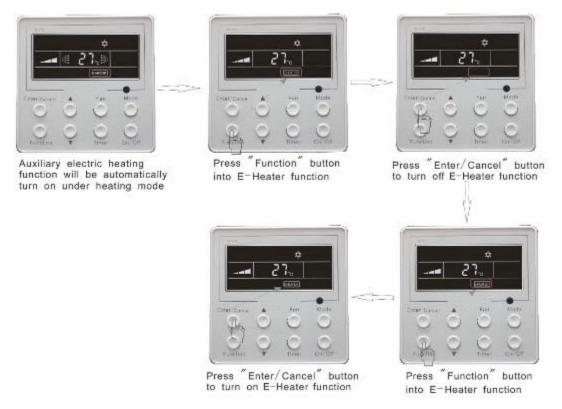
Fig. 5.11 Auxiliary Electric Heating Function Setting
