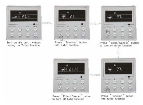
Fig.5.9 Turbo Function Setting
