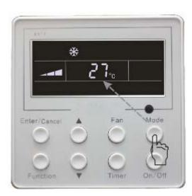
Press ▲ or ▼ button for increase or decrease of setting temperature under on state of the unit.
