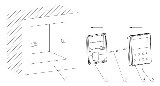
Fig.4.1: Sketch for Installation of Wired Controller
