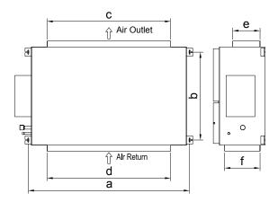
Fig. 19 Indoor unit installation position and dimension
