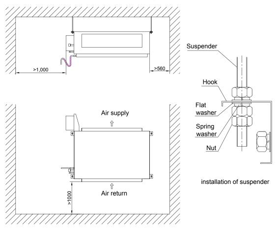
Fig.20 Schematic for the indoor unit
