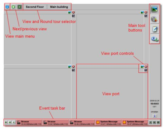
The view ports fill the central part of the window, and each view port has its own view port controls.
