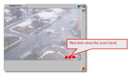
**Please note:** When PTZ control is enabled, any mouse actions are taken for PTZ control. In order to control the client-based view port zooming (see *6.2.3 Zooming in a view port and in archive recordings* on page 51), hold down the **CTRL** key while using the mouse.
