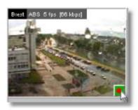
You can switch recording on and off by pushing the manual recording button. The recording state is shown by the color (a strong red dot means recording is on, otherwise recording is off).
