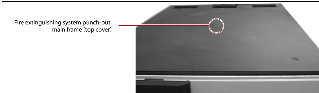
Figure 12 Location of the fire extinguishing system access opening in the top of the library.
