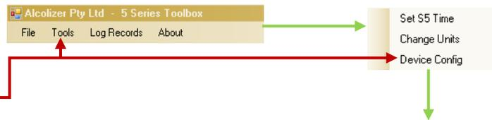
**Download From Device** This function downloads the present S5 device configuration into the **Configuration Editor** display window.
