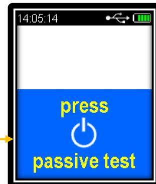
2. Press **TEST**
