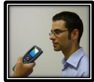
*Note: The device is set to take 3 pump samples. During these 3 pumps the operator must hold the device steady and at the same distance from the subject. The 5 Series will give 3 sample pump clicks, followed by a long beep sound. Analysing Sample will then appear.*
