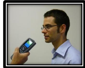
*Note: The device is set to take 3 pump samples. During these 3 pumps the operator must hold the device steady and at the same distance from the subject. The 5 Series will give 3 sample pump clicks, followed by a long beep sound. Analysing Sample will then appear.*
