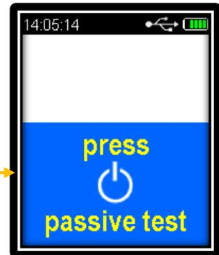
2. Press **TEST**
