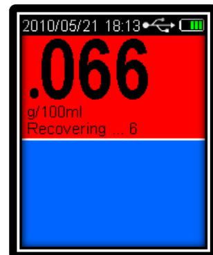
When **Recovery** period has elapsed the device is ready for next passive breath test. The BAC display window will be clear if "**Keep Previous Reading**" function was not enabled.
