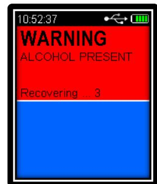
When **Recovery** period has elapsed the device is ready for next passive breath test. The BAC display window will be clear if "**Keep Previous Reading**" function was not enabled.
