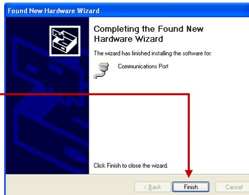
*Note: Every time you connect to a new USB connection port that has not had the Series 5 USB driver previously installed, the above “Found New Hardware” installation process will be repeated.*
