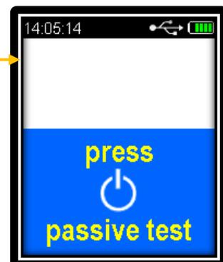
*Note: If the device function “Keep Previous Reading” is enabled, the last passive reading is retained on the display screen until another passive breath test procedure is started.*
