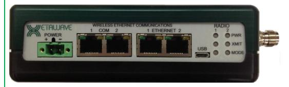
The right side of the radio has one or two female TNC connectors for the one internal radio in Xeta9-E or two internal radios in Xeta9x9-E. Radio #1 is the connector closest to the front of the radio.
