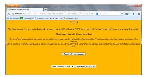
5. Next, enter the radio's new IP address in the address bar of your web browser and load the page. Note: Depending on your computer's configuration, it may be necessary to change or add an IP address on your computer to be on the radio's new subnet.
